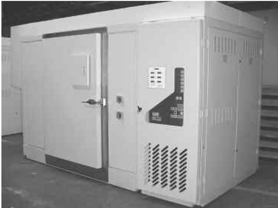
Most of the control devices are contained within three sections in the service compartment inside the front RHS of the chamber.
