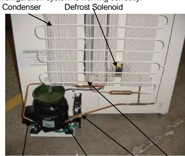
Condenser Defrost Solenoid Cooling fan CPR Valve
