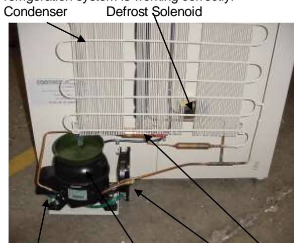
Suction line Compressor Cooling fan CPR Valve
