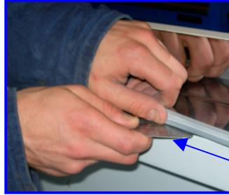
Special flat tool to push the seal under the facia
