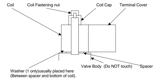
The Contherm Part No for the washer is: WASHER 29 This is a 1/2" 1mm thick steel washer.
