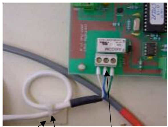
'Sticky Pad' Cable tie PCB Connector
